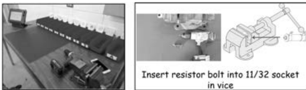
Fig. 1. a. Prototype of the workstation to help trainees assemble an electrical resistor. b. PowerPoint slide showing one adapted instruction to facilitate assembly.
